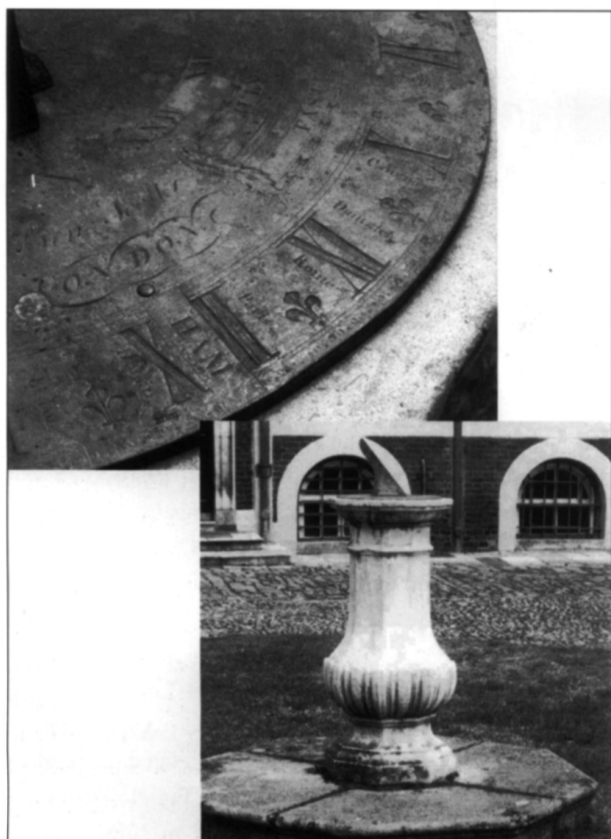
Fig.2. A Benjamin Scott dial at Ham House, Richmond. Note the names of places next to the hour numerals, including "HAM" in the noon gap. Photos: P. Powers.
