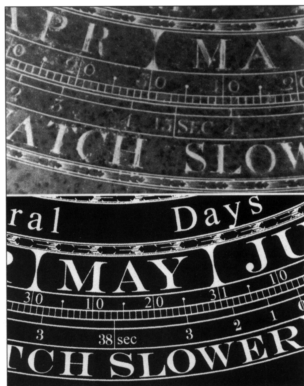
Fig.9. An example of the Equation of Time ring on Grocers' pattern dials. The upper picture is of the Suffolk Adams dial; the lower one is from a modern reconstruction. Note the difference in the data of the maximum value due to the calendar change and also the different value due to changes in the longitude of perihelion.
